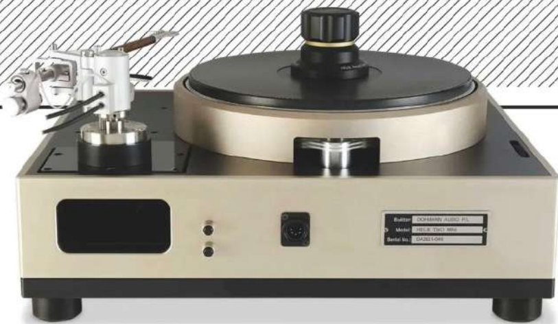
ABOVE: Rear view shows the double-belt drive system, 5-pin PSU connector and up/down buttons for the Helix Two's fine speed control. The void under the armboard [left] allows tonearm leads to be 'dressed' without compromising the suspension
